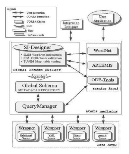
Fig. 2. The architecture of the *MOMIS* system
